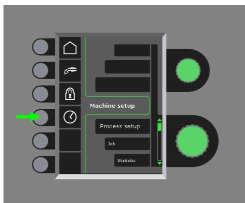
It is important to set the correct time, if logging of e.g. errors should be used. The setting is confirmed by pressing the following key pad after the setting is completed:
