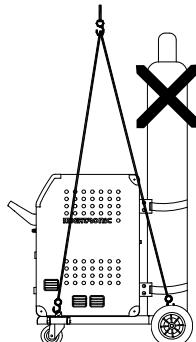
Do not lift the machine by the handle.
