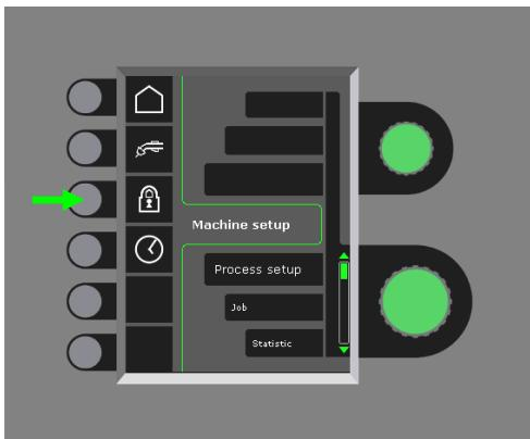
Functions are locked to the selected lock level by inserting the SD-lock-card and unlocked by reinserting the SD lock-card.
