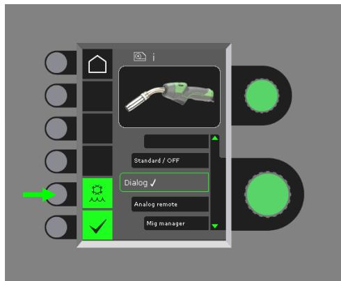
When a MIG Manager® is connected, it will automatically control the water cooling function and disable this configuration.
