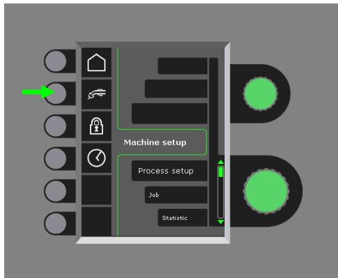
Turn the lower control knob until the requested configuration is displayed. Press the ✓-knob to confirm the selection (selected configuration is indicated by ✓):
